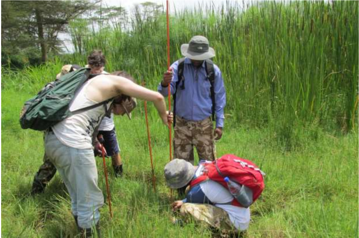
Figure 2.1: Assessing the sediment depth at Ormakau using metal rods to reach the bedrock under the swamp sediments. Photograph: Rebecca Muthoni, 30 March 2013.
