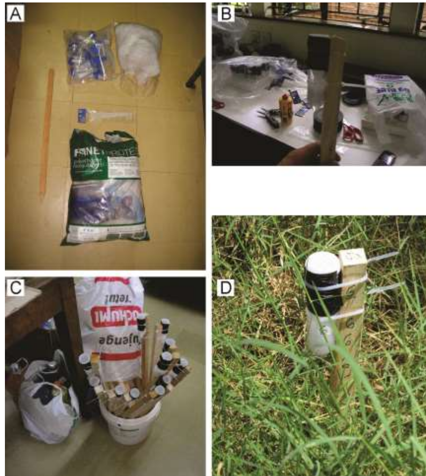
Figure 2.5: A) Main components of the Behling design pollen traps (Behling et al. , 2001; Jantz et al. , 2013), B) a completed trap, C) traps were shipped from the National Museums of Kenya covered in plastic, and D) a deployed trap at Kimana Swamp location 6. Photographs: A-C Colin Courtney Mustaphi and D Esther Githumbi.
