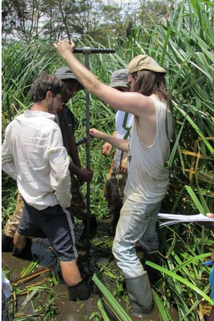
Figure 2.2: Collecting deep sediments from Ormakau using a Russian Corer with extension rods. Photograph: Esther Githumbi, 31 March, 2014.
