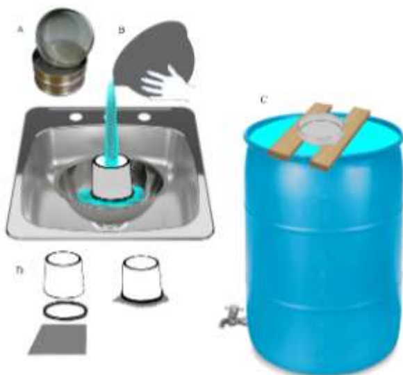
Fig. 10. Washing in the lab. (A) Laboratory soil sieves are good for the lab but too small for the field. (B) Protecting sink from the sediment. (C) Washing barrel. (D) Small sieve with removable nylon net.
