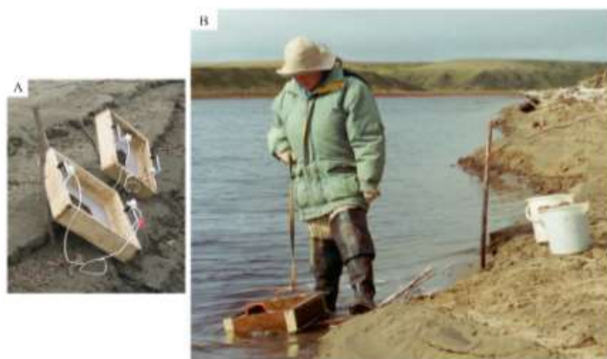
Fig. 4. Rope or belt help to change working position. (A) Sieves with ropes. (B) S. Kuzmina is screening at the Lena River Delta.
